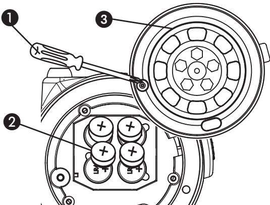
**Note:** To remove batteries, insert a screwdriver (or similar tool) into the recessed area of each battery well and gently lift the battery from the well.
