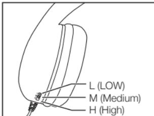
The volume switch is located on the inside of the left ear cup. Before use, have an adult use the tip of a pencil, paper clip, or other small tool to slide the switch to set the headphone volume to High, Medium or Low.
